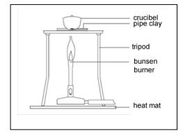
The student strongly heated a 4.00 g sample of  $CuSO_4$ .xH<sub>2</sub>O and recorded the mass of the sample every two minutes to constant mass. The final mass recorded was 2.65.
